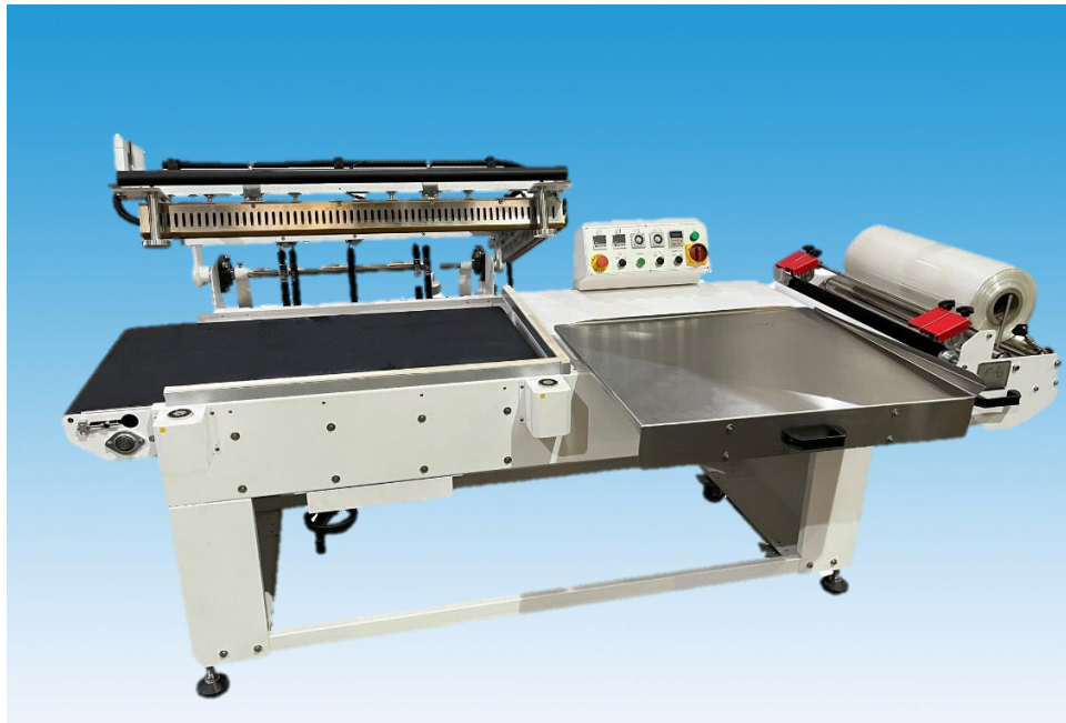
Advanced sealer blade design and independent heat control for each blade for smoke free operation
